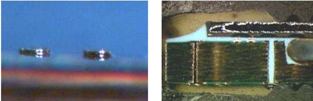
Figure 14, a) coined stud bumps (picture courtesy of Microemissive Displays) b) investigation of underfill flow between a substrate and die containing an open cavity
