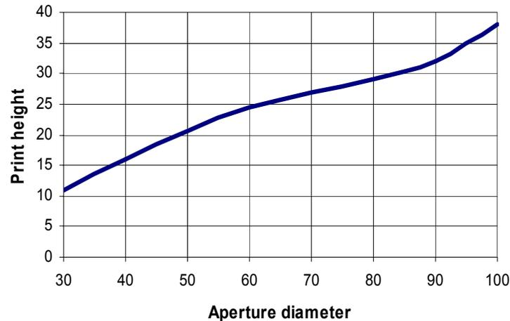
Figure 12 Aperture diameter vs. print height
