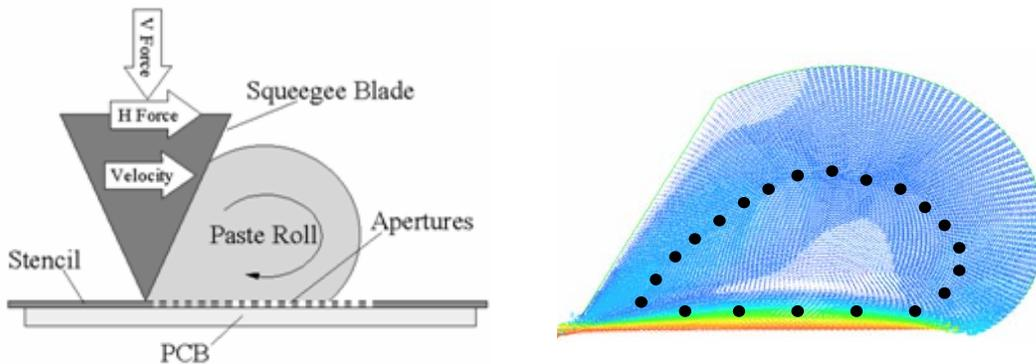
Figure 8, a) schematic of paste roll b) Results of velocity vectors using Non-Newtonian CFD
