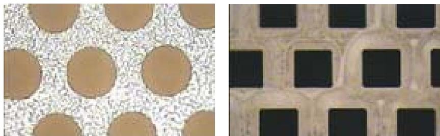
Figure 3, a) rough upper stencil surface, b) smooth upper stencil surface
