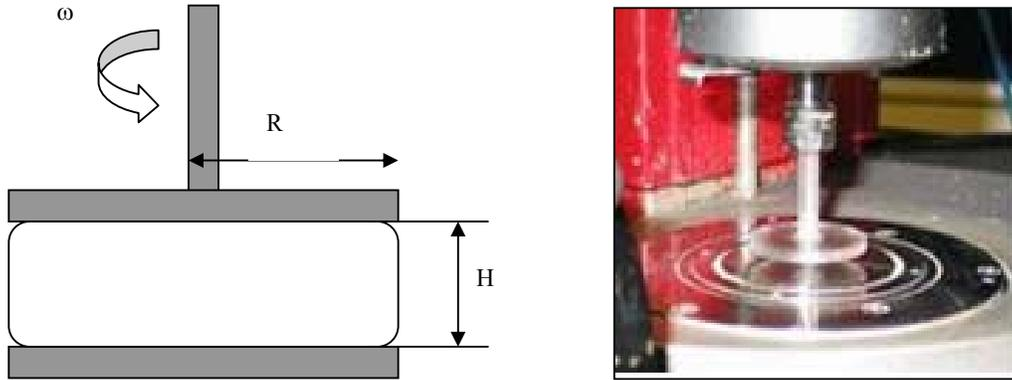
Figure 6, Stress and strain rheometer test
