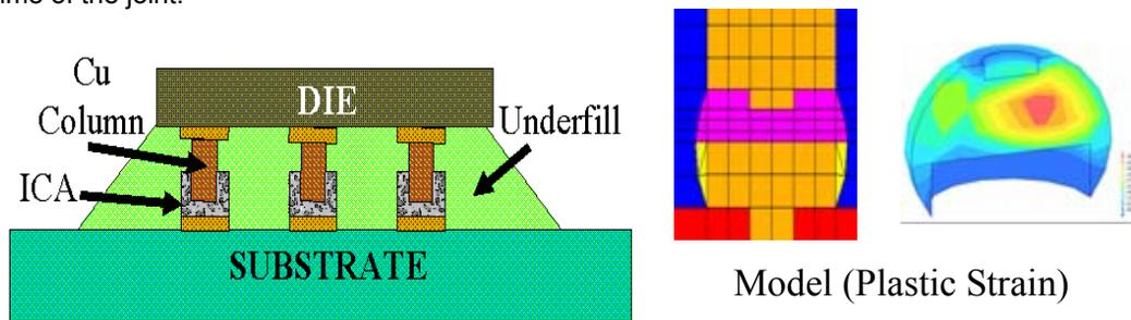
Figure 13, a) Flip-chip assembly under investigation b) Modeled results of Plastic Strain
