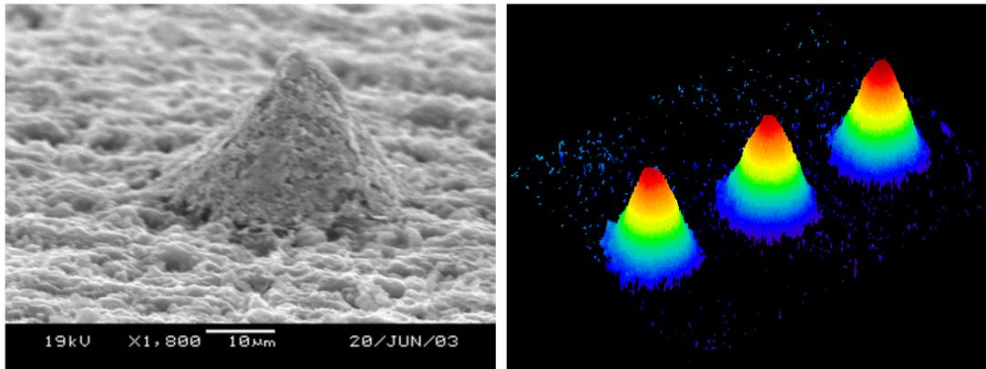
Figure 11, Side profile of adhesive deposit
