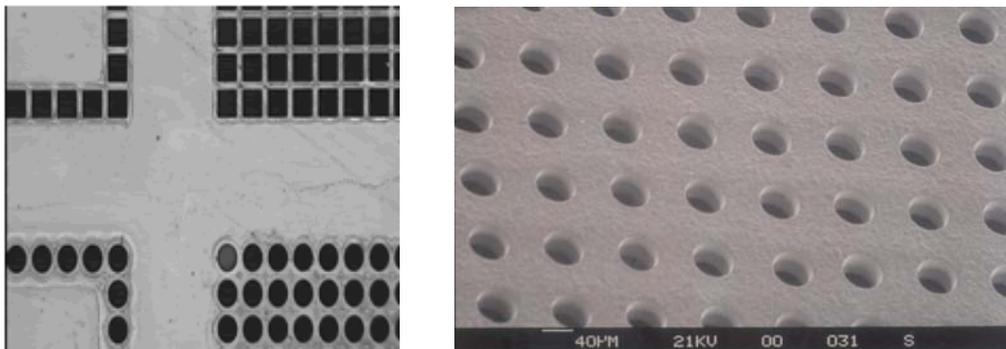
Figure 2, Microengineered stencil a) optical image of square and oval shape apertures at  $90\mu\text{m}$  pitch
