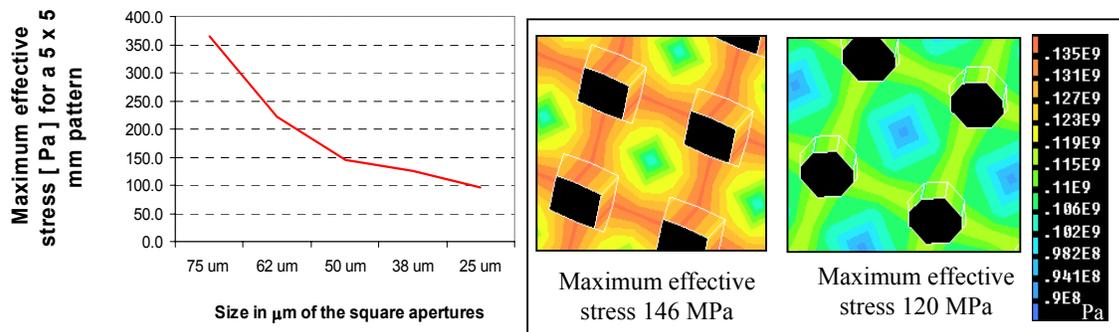
Figure 5, a) Stencil stress as function of aperture size b) stress as a function of aperture shape
