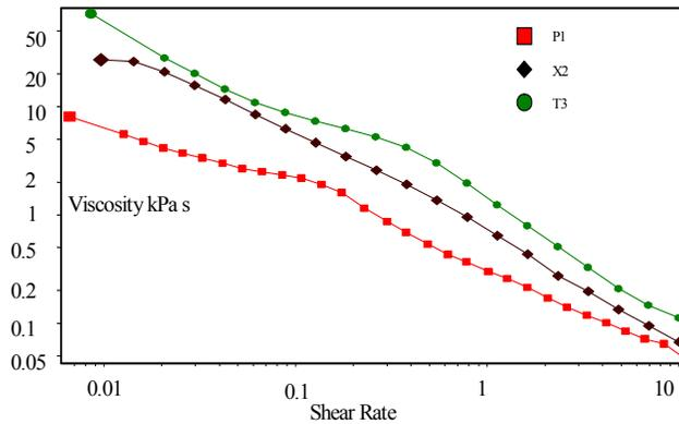
Figure 7 Viscosity vs. shear rates (1/s)
