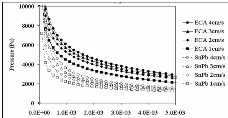
Figure 9 Pressure in paste material at different distances from blade tip
