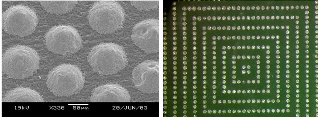
Figure 10, a) SEM Image of 90 $\mu\text{m}$  pitch adhesive print deposits b) Optical image of 100 $\mu\text{m}$  pitch adhesive print deposits
