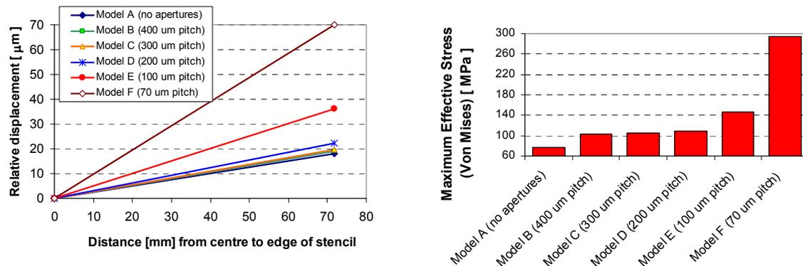
Figure 4, a) Stencil deformation vs. aperture pitch b) stress as a function of increasing pitch
